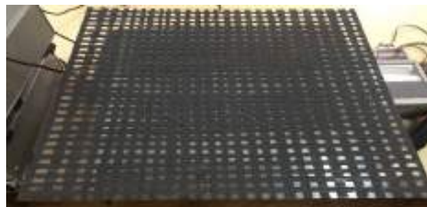
Fig. 2. Orthogonal grid with graphite powder strips
