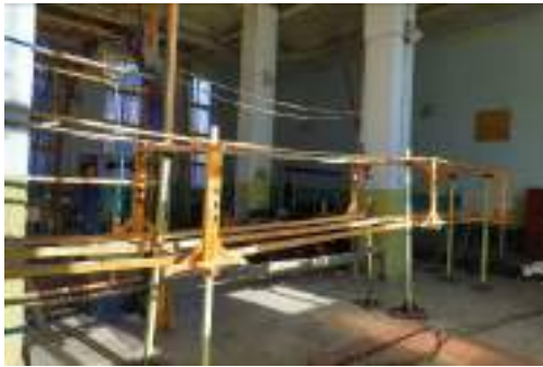
Fig.1. The laboratory model of a single-circuit overhead power transmission line with a triangular arrangement of wires
