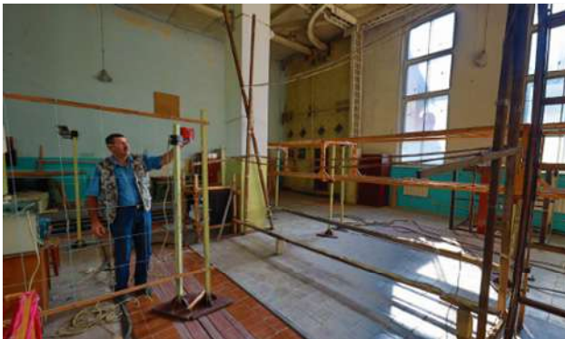
Fig. 13. Picture of three shielding coils spatial arrangement of system of active shielding laboratory model
