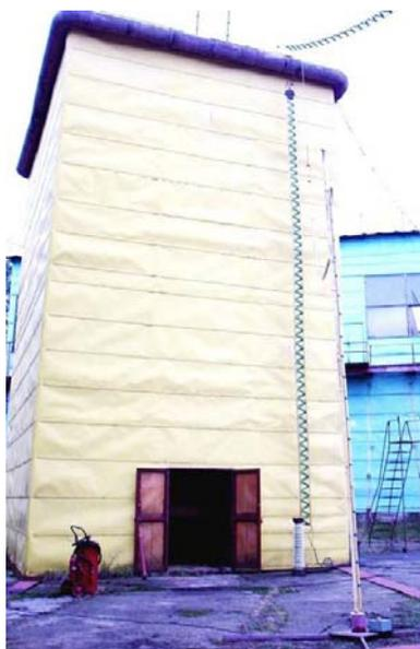
Fig. 2. External view of the modernized powerful ultra-high-voltage high-current generator of the GINT-2 type, containing a flat steel shield-roof with slope of rectangular shape with area of  $60 \text{ m}^2$  with round edges (in the foreground, to measure the ATPs of voltage pulses formed at the test object, an ohmic voltage divider is installed on  $\pm 2.5$  MV of the ODN-2 type)
