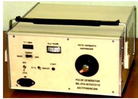
Fig. 16. Generator of type TI-CS115 (NCS08), which reproduces pulse currents of the form CS115 [9] and NCS08 [7] on the TO
