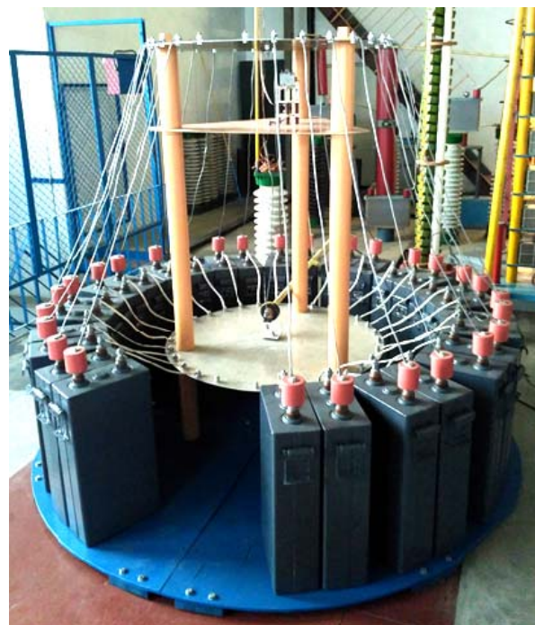
Fig. 25. General view of a high-voltage current pulse generator of the G-NCS10 type, which implements the requirements of the NATO AESTR-500: 2016 Standard when testing OAMT in the form of NCS10 (Scientific-&-Research Planning-&-Design Institute «Molniya» of NTU «KhPI», Kharkiv, 2018)
