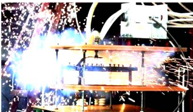
Fig. 10. Results of the electrothermal action in the discharge circuit of the GTM-10/350 type artificial lightning current generator of a normalized aperiodic current pulse of a short thunderstorm discharge of a temporary shape of 17/265 \mu\text{s} with amplitude of I_m \approx -83.8 \text{ kA} on the test sample of the АППВНГ2×6 network cable with PVC insulation and solid aluminum core of cross section of 6 \text{ mm}^2 [23]
