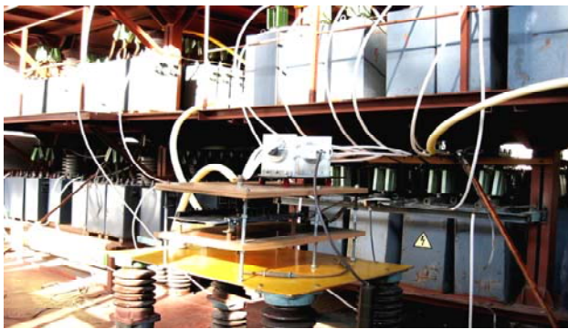
Fig. 7. General view of a powerful high-voltage high-current generator of artificial lightning type GTM-10/350 (in the foreground there is its desktop with a controllable high-voltage three-electrode air switch placed on top of it with graphite electrodes for voltage \pm 50 \text{ kV} and pulsed aperiodic lightning current with amplitude up to \pm 220 \text{ kA} and a test sample of cable and wire products, and in the background there are the electrical elements of the charge-discharge circuits of its individual high-voltage pulse current generators GIT-1, GIT-2, GIT-3 and GIT-4) [21]
