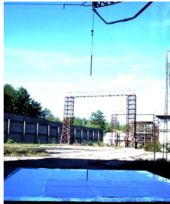
Fig. 14. General view of the TO – a two-electrode needle-plane system with an air gap of 3 m, to the upper electrode of which GKIN-2 and the measuring ohmic divider of the pulse voltage ODN-2 to rated voltage of \pm 2.5 MV are galvanically connected [29]
