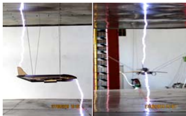
Fig. 26. Frames from the process of experimental determination of the likely places of a lightning strike in an airplane model
