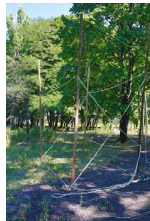
Fig. 10. Picture of both shielding coil spatial arrangement of system of active shielding model
