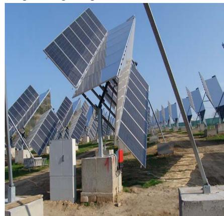
Fig. 1. Example of SGM module, equipped with a one-sided low solar concentration system
