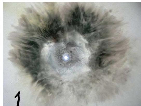
Fig. 16. General view from the binding zone on the outer surface of the TS of a flat duralumin panel ( $h=1.2$  mm) of the aircraft's fuel tank of the plasma channel simulated by the UITOM-1 installation of a lightning discharge of the results of direct exposure to this TS for zone 1A of the normalized components of the artificial lightning current, characterized by through local penetration of the TS panel wall at the point of impact of the lightning channel
