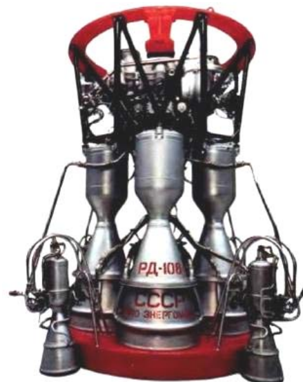
Fig. 6. Four-chamber LRE of PД-108 type used at the second stage of the Soviet P-7 (8K71) ICBM [22]
