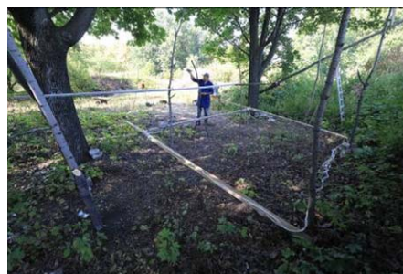
Fig. 6. Picture of the shielding coil (a) and the experimental isolines of the resultant magnetic flux density with the systems of active shielding is on (b)
