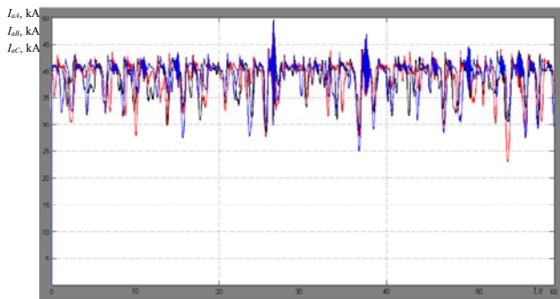
Fig. 5. Temporal dependencies of the arcs currents of the furnace ДСП-200 with the regulation by the obtained model (4) of minimizing the dispersion of the three-dimensional vector of arcs currents in the two-contour structure of the ACS of the EM of the arc furnace ДСП-200
