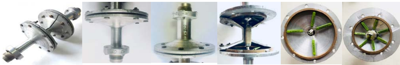
Fig. 2. Photo of autonomous resistive shielded low-resistive voltage divider (ARSLVD)
