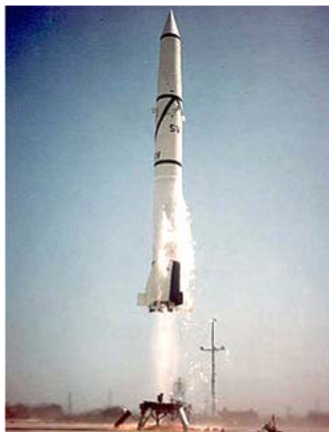
Fig. 4. The start of the Redstone medium-range ballistic missile (length – 21.1 m; diameter – 1.78 m) with a detachable warhead created in the USA under the scientific and technical guidance of Wernher von Braun [11]
