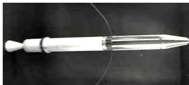
Fig. 5. External view of the first American artificial satellites Explorer-1 (1958, gross weight – 14 kg, USA) [14]
