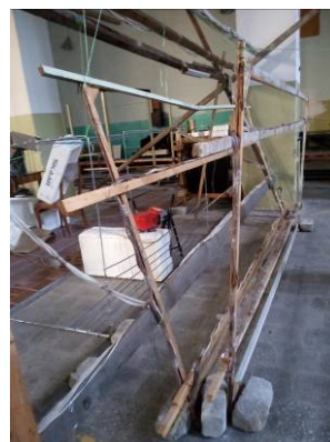
Fig. 12. Two compensating windings of active shielding system
