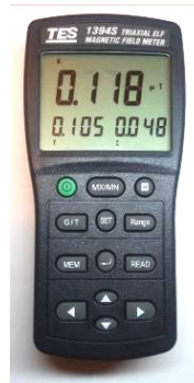
Fig. 9. Three-coordinate magnetometer for measuring resulting magnetic field
