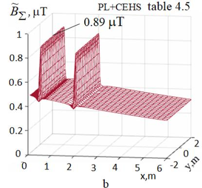
Fig. 5. Total minimum (a) and maximum (b) influences of the PL+TS to the level  $\tilde{B}_\Sigma$
