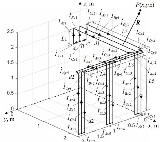
Fig. 2. The investigated low-voltage busbar TS 100 kVA 6(10)/0.4 kV
