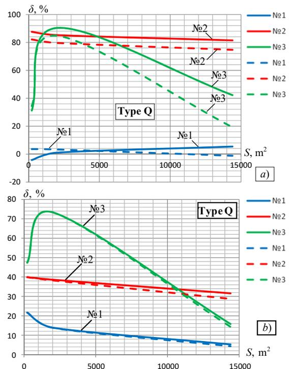
Fig. 3. Error in determining normalized parameters depending on the area of the GD and the method of equivalence of soil type Q: a – solid curve –  $U_{ic}$ ; dotted curve –  $U_{ik}$ ; b – solid curve –  $R_G$ ; dotted curve –  $U_G$
