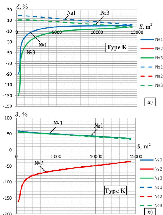
Fig. 4. Error in determining normalized parameters depending on the area of the GD and the method of equivalence of soil type K:
