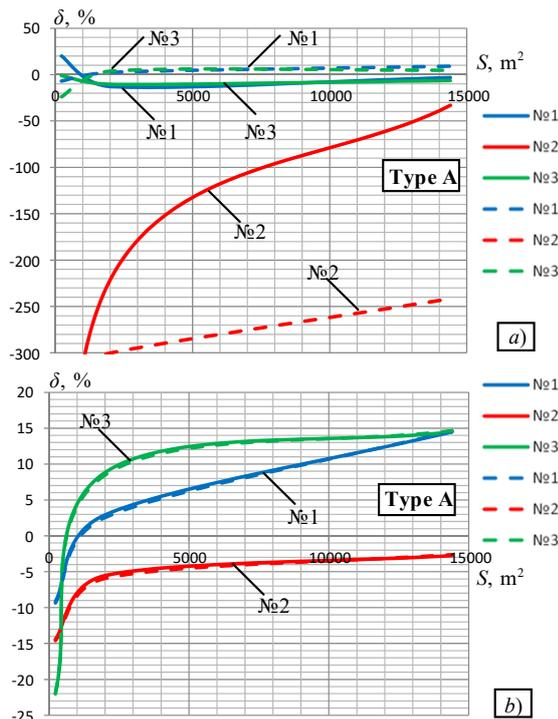
Fig. 1. Error in determining normalized parameters depending on the area of the GD and the method of equivalence of soil type A: a – solid curve –  $U_{ic}$ ; dotted curve –  $U_{ik}$ ; b – solid curve –  $R_G$ ; dotted curve –  $U_G$
