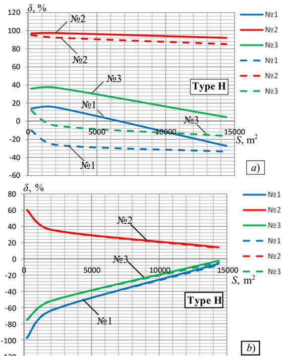
Fig. 2. Error in determining normalized parameters depending on the area of the GD and the method of equivalence of soil type H: a – solid curve –  $U_{ic}$ ; dotted curve –  $U_{ik}$ ; b – solid curve –  $R_G$ ; dotted curve –  $U_G$
