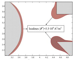
Fig. 11. Isodines  $F^*| = \text{const}$  and their corresponding extraction domains of the force field at  $|F^*|_{\text{min}} = 5.5 \cdot 10^9 \text{ A}^2/\text{m}^3$ for a fragment of the matrix working space
