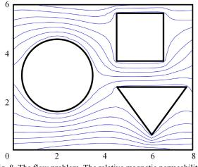
Fig. 8. The flow problem. The relative magnetic permeabilities of discrete elements  $\mu = 1$ , of the external medium  $\mu_e = 1000$
