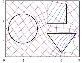
Fig. 7. Relative magnetic permeabilities of triangular, square and round rods, respectively, equal to 1000, 10 and 2,  $\mu_e=1$ . The external field  $H_0$  is directed at an angle of 45° to x-axis
