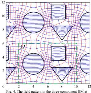
relative magnetic permeabilities of discrete elements  $\mu$ =1000 and the external medium  $\mu_e$ =1. Green dotted line illustrates the main parallelogram of the periods. External field  $H_0$ =1
